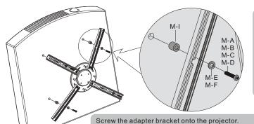
Note: If there are only three mounting holes using three arms of adapter bracket.
