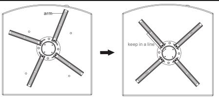
Place the projector bracket as close as possible to the projector's center of gravity. Position the holes of arms over the mounting holes.
