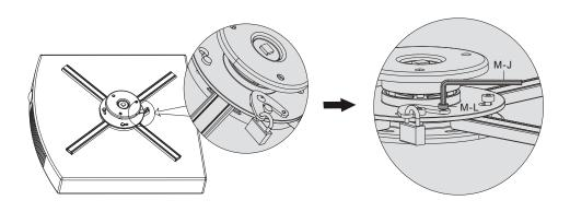
Use the padlock in the locking plate and then fix the locking plate with a screw to prevent the projector plate assembly rocking in use.
